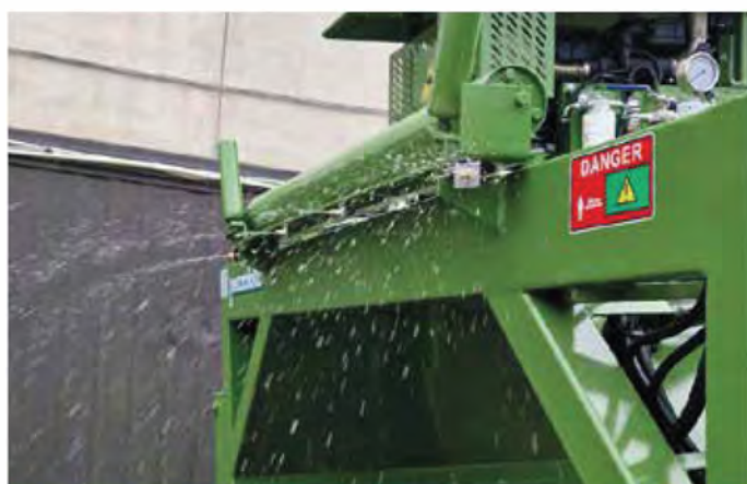
Two-inch ramp for liquids distribution
