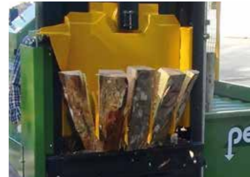
VS 60 - Bowed wedge with 4 orbital knives
