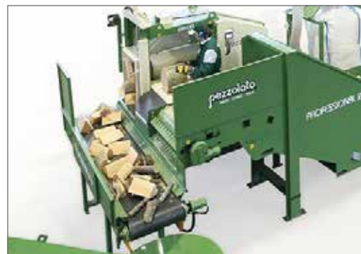
Flat conveyor for one splitting station
