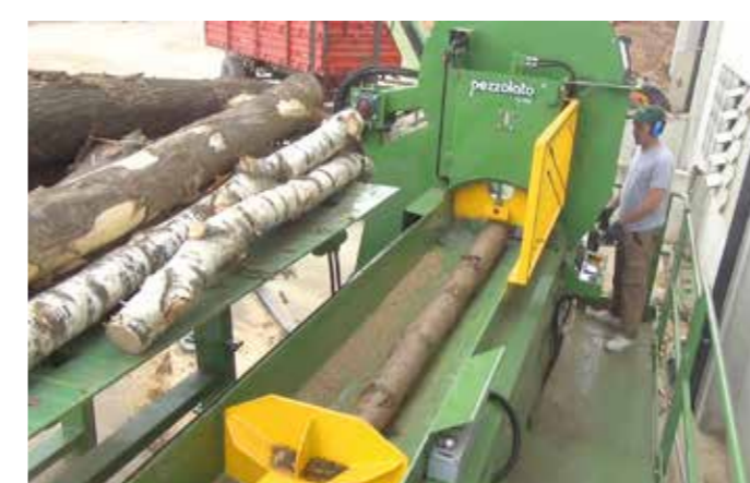
Feeding conveyor and wood pusher (TLF model)
