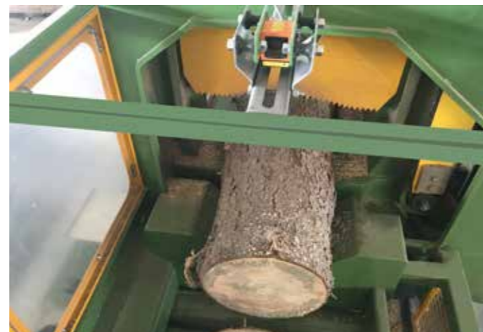
Photorelay for automatic log length measurement
