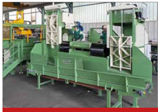
Flat conveyor for two splitting stations
