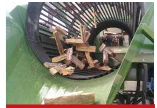
Output logs without bark and residual sawdust
