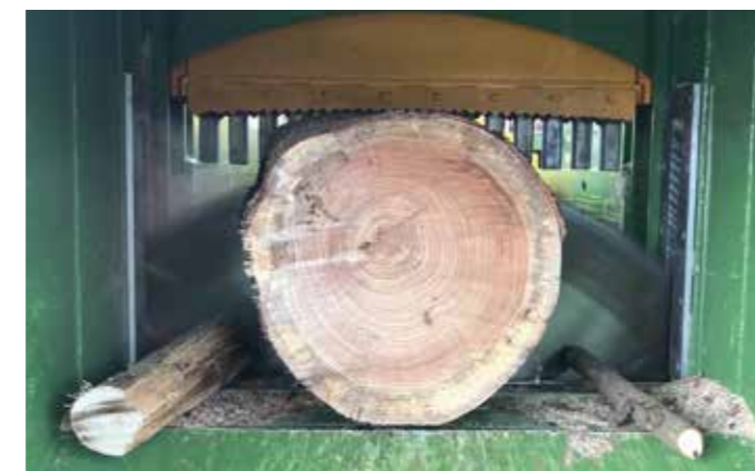
Feeding with large diameter logs (TLA)
