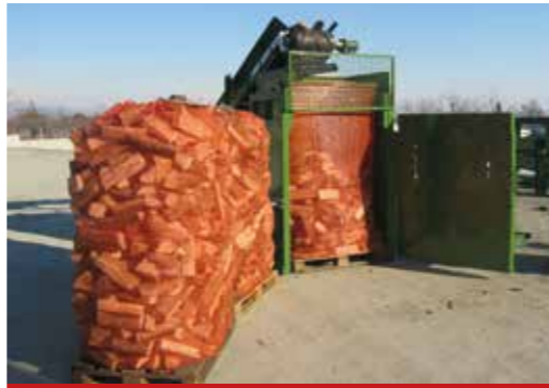
Pallet packer with electric motor drive
