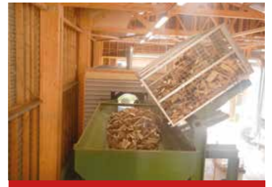
Drum screener with feeding hopper
