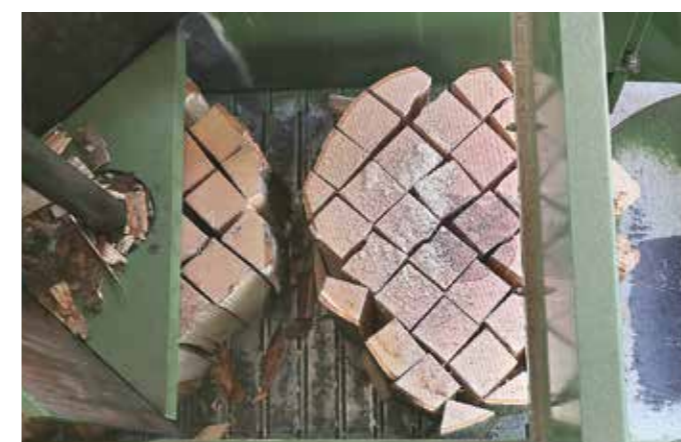
Wedge for automatic vertical splitting system
