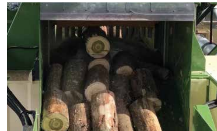
Mechanical jacks locking system. Efficient on all species of bundles
