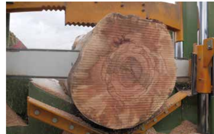
Horizontal sliding cut-off chain
