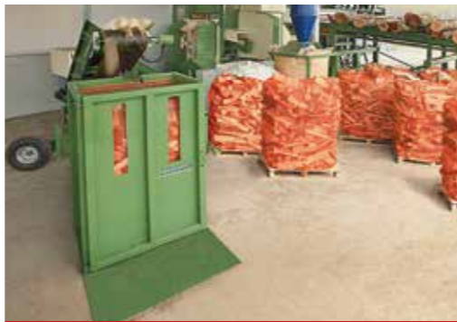
Pallet packer with machine hydraulics drive
