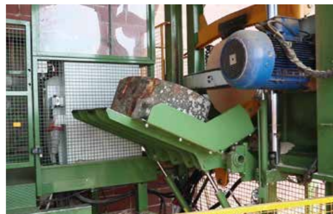
Tilting surface for for offloading cut logs
