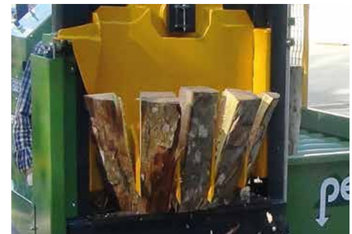
Wedge with 4 orbital blades producing 5 logs per cycle
