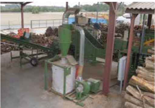
Aspirator with collecting system in "big bags"
