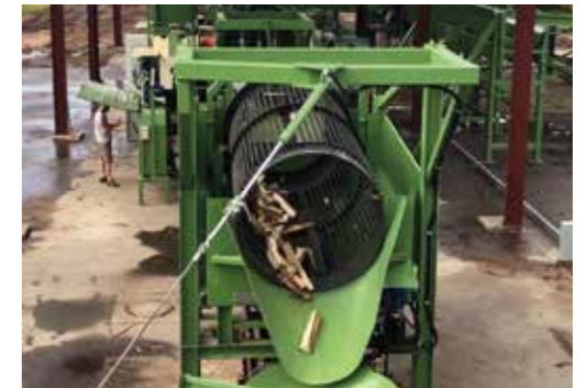
Drum screener with 1800 mm drum diameter
