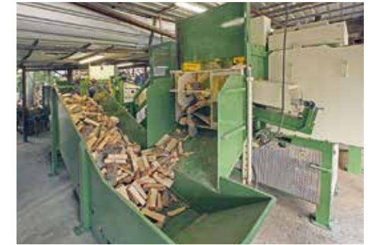
S-shaped conveyor combined with TLC 1200
