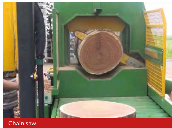
Motorized rollers table for transferring cut logs
