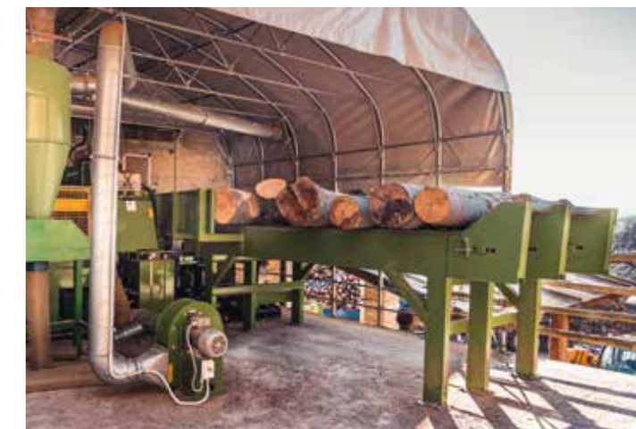
3-chain loading deck, 4 meters in length
