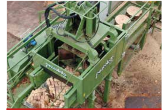
Automatic vertical splitter TB 900
