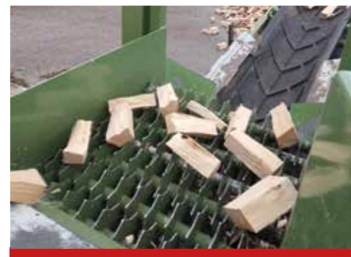
Cleaning rollers combined with TB 900
