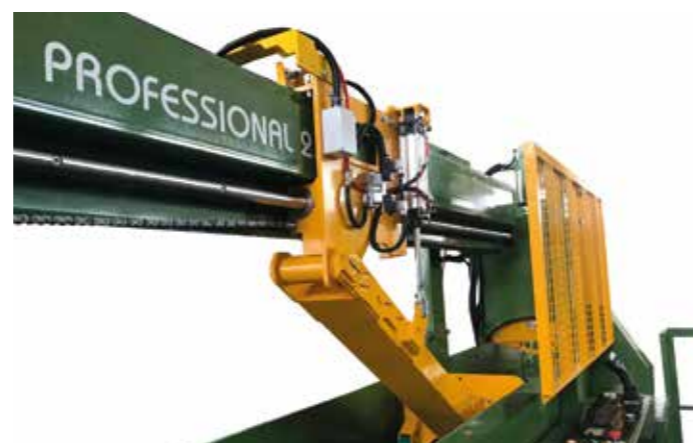
Lifting pusher with mechanical/pneumatic system
