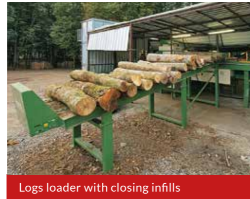
Logs loader with log separating system
