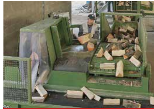
11 Ton splitting station, 2+4 folds grid
