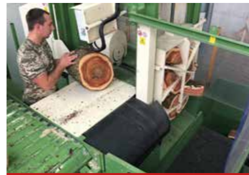
20 Ton splitting station, 2+4+6 folds grid
