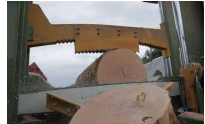
Wood clamping hydraulic guillotine
