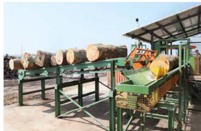
Feeding cradle with rear pushing unit
