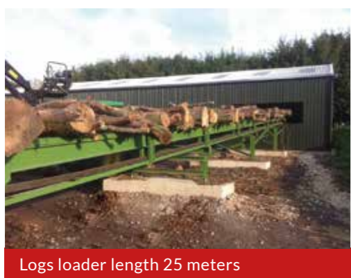
Loading system with pusher
