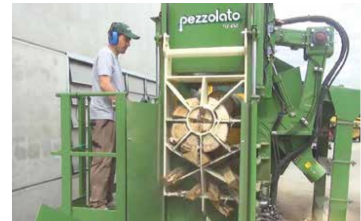
Adjustable splitting grid (TLF model)
