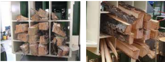
GENIUS WEDGE splitting grid designed to obtain the firewood calibration in one single step, optimising logs diameter and minimising waste
