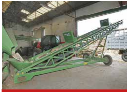
Driven caster wheels hydraulically operated
