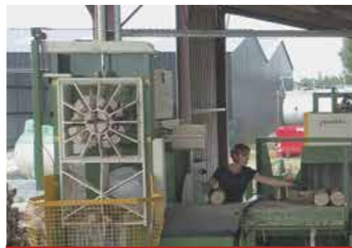
32 Ton splitting station, 2+4+6+16 folds grid
