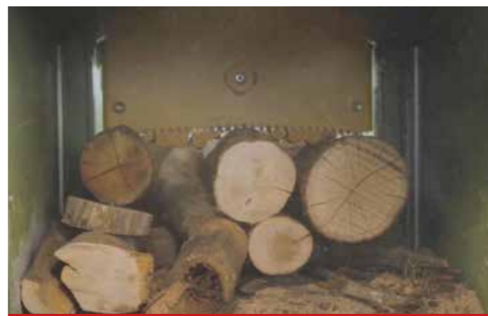
Hydraulic chain wood blocking
