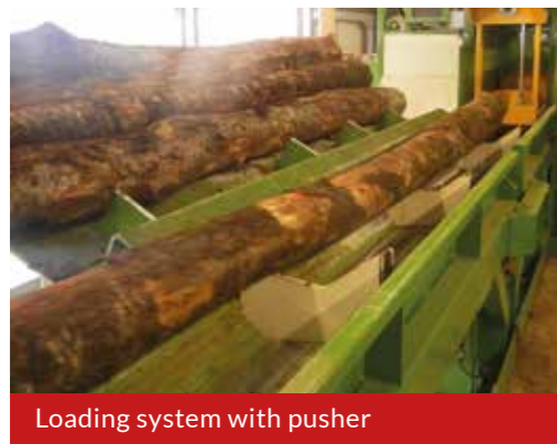
C-shaped loading system
