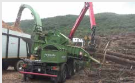
Machine with angled hopper
