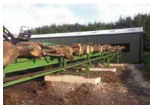
Ladestation 25 m lang, 4-strangig
