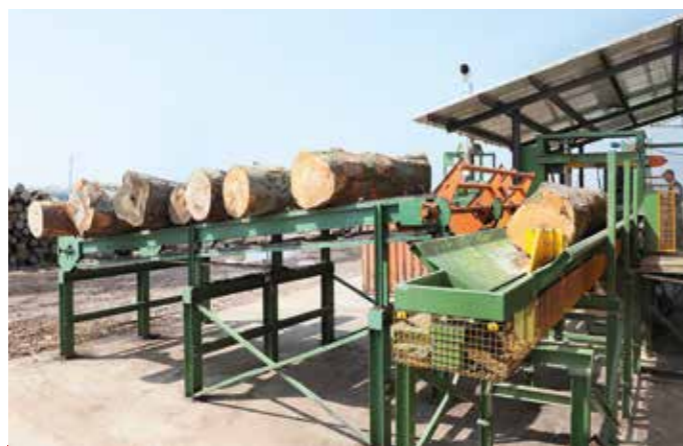
Feeding cradle with rear pushing unit
