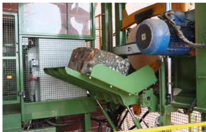
Tilting surface for for offloading cut logs
