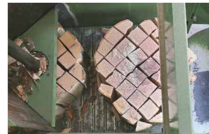
Wedge for automatic vertical splitting system
