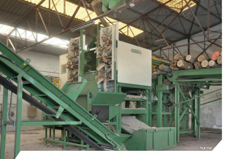
Then, once again automatically, the mesh containers are filled with the clean material and carried to the drying cells. Once the right degree of moisture has been reached, these containers are emptied out into a vibrating chute that feeds a second screen to further remove impurities from the wood as it is being dried, before moving on to packaging. In 3 shifts of 7 hours, each system produces over 90,000 tons of finished material per year.
