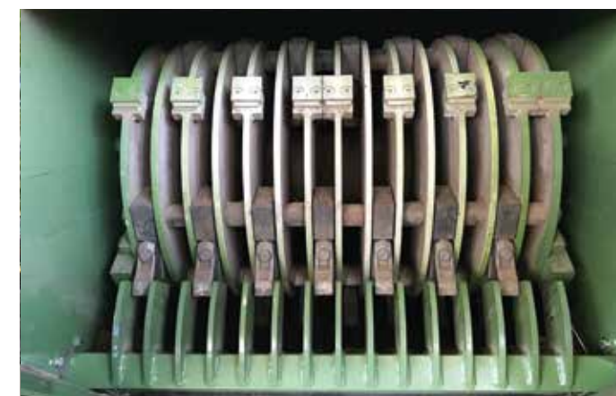
Rotor S 10000 with mobile hammers with counter-hammer
