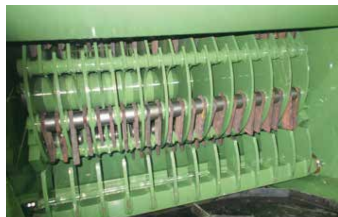
Rotor S 9000 with mobile hammers with counter-hammer
