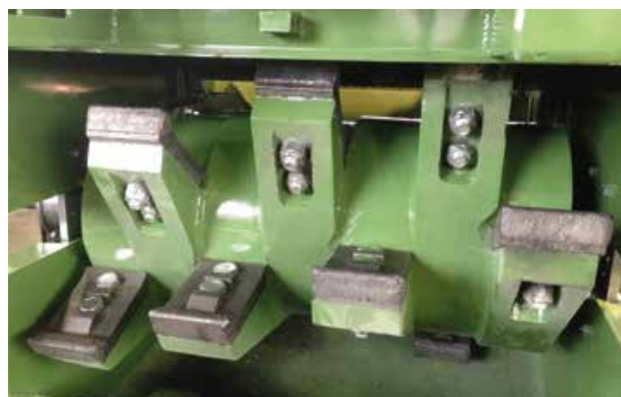
Rotor S 10000 with fixed hammers
